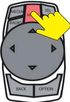
Long press MENU key to switch between OEM system and ANDROID system.
